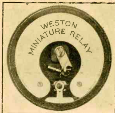
Sensitive milliammeter designed to work with electronic tubes. 200 microamperes applied to this relay will close contacts permitting up to 30 milliamperes, to flow in a local circuit.
